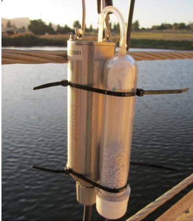
**Figure 6.** Desiccant tube fix against atmospheric pressure effect
